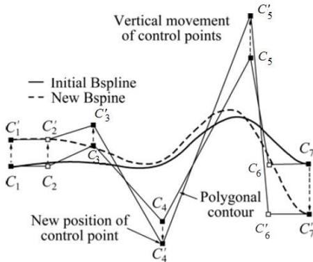
Figure 1. B-Spline curves defining the preform shape.
