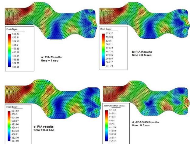
Figure 1. Comparison between PIA and ABAQUS<sup>®</sup>.
